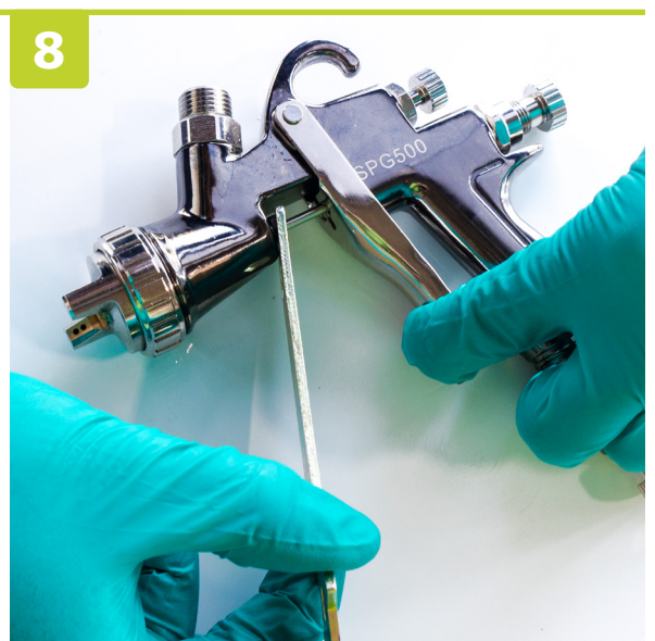
8 • Tighten screw until needle doesn't move • Gently loosen the screw until the needle moves fluently again.
