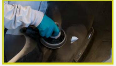
**05** APPLY THE PLASTIC REPAIR WITH THE GUN ON THE REINFORCEMENT CANVAS Keep nozzle in product to prevent air bubbles
