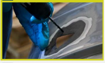
**06** PRESS THE PRODUCT FROM THE INSIDE OUT TO THE AESTHETIC SIDE OF THE REPAIR SPOT THRU THE HOLES.
